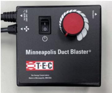
Each system comes with one fan speed controller. Fan speed is adjusted using the adjustment knob on the face of the fan speed controller or by connecting to the DG-1000 for Cruise Control.
