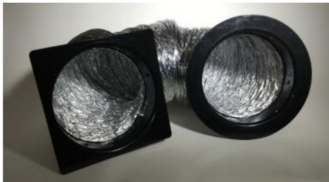
The flexible extension duct consists of a 12 foot long section of 10" round flexible duct with one square and one round black plastic transition piece attached at either end.
